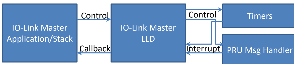
Figure 3 : IO-Link Master Interrupts and Controls
